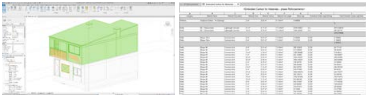
Caption: Revit was used to semi-automate embodied carbon calculations
